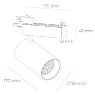
COB 4200 [K] MEAT WHITE Light colour CRI 90 Led chip flux 1976 [lm] Luminous flux 1580 [lm] System power 19 [W] Luminaire Efficiency 83 [lm/W] Beam angle 30° Controller ON/OFF MacAdam 3 SDCM
