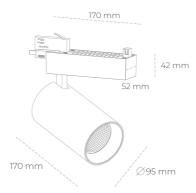
COB 4200 [K] MEAT WHITE Light colour CRI 90 Led chip flux 2159 [lm] Luminous flux 1727 [lm] System power 21 [W] Luminaire Efficiency 82 [lm/W] Beam angle 15° Controller ON/OFF MacAdam 3 SDCM
