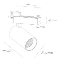
COB 4200 [K] MEAT WHITE Light colour CRI 90 Led chip flux 1412 [lm] Luminous flux 1129 [lm] System power 14 [W] Luminaire Efficiency 81 [lm/W] Beam angle 15° Controller ON/OFF MacAdam 3 SDCM
