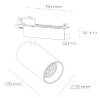
COB 4000 [K] HI EFFICIENT Light colour CRI 90 Led chip flux 4385 [lm] Luminous flux 3508 [lm] System power 27 [W] Luminaire Efficiency 130 [lm/W] Beam angle 15° Controller ON/OFF MacAdam 3 SDCM
