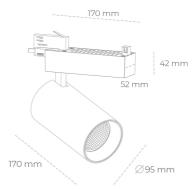
COB 3500 [K] HI EFFICIENT Light colour CRI 90 Led chip flux 4181 [lm] Luminous flux 3344 [lm] System power 27 [W] Luminaire Efficiency 124 [lm/W] Beam angle 45° Controller ON/OFF MacAdam 3 SDCM
