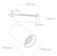
COB 3500 [K] HI EFFICIENT Light colour CRI 90 Led chip flux 4723 [lm] Luminous flux 3778 [lm] System power 31 [W] Luminaire Efficiency 122 [lm/W] Beam angle 30° Controller ON/OFF MacAdam 3 SDCM
