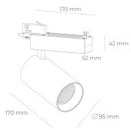
COB 3500 [K] HI EFFICIENT Light colour CRI 90 Led chip flux 2174 [lm] Luminous flux 1739 [lm] System power 14 [W] Luminaire Efficiency 124 [lm/W] Beam angle 30° Controller ON/OFF MacAdam 3 SDCM
