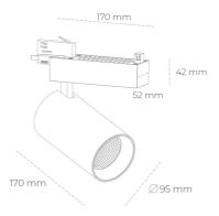
COB 3500 [K] HI EFFICIENT Light colour CRI 90 Led chip flux 2174 [lm] Luminous flux 1739 [lm] System power 14 [W] Luminaire Efficiency 124 [lm/W] Beam angle 15° Controller ON/OFF MacAdam 3 SDCM
