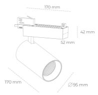
COB 3000 [K] HI EFFICIENT Light colour CRI 90 Led chip flux 3487 [lm] Luminous flux 2789 [lm] System power 21 [W] Luminaire Efficiency 133 [lm/W] Beam angle 45° Controller ON/OFF MacAdam 3 SDCM
