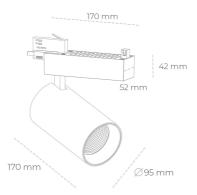
COB 3000 [K] HI EFFICIENT Light colour CRI 90 Led chip flux 4956 [lm] Luminous flux 3964 [lm] System power 31 [W] Luminaire Efficiency 128 [lm/W] Beam angle 15° Controller ON/OFF MacAdam 3 SDCM
