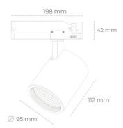
COB 2000 [K] MEAT PINK Light colour CRI Led chip flux 2013 [lm] Luminous flux 1610 [lm] System power 23 [W] Luminaire Efficiency 70 [lm/W] Beam angle 60° Controller ON/OFF
