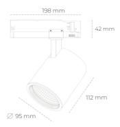
COB Light colour 2000 [K] MEAT PINK CRI Led chip flux 2013 [lm] Luminous flux 1610 [lm] System power 23 [W] Luminaire Efficiency 70 [lm/W] Beam angle 15° Controller ON/OFF MacAdam 3 SDCM
