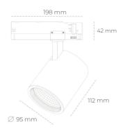
COB 3000 [K] CRI97 Light colour CRI Led chip flux 2990 [lm] Luminous flux 2392 [lm] System power 27 [W] Luminaire Efficiency 89 [lm/W] Beam angle 45° Controller ON/OFF MacAdam 3 SDCM
