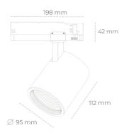
COB 4000 [K] HI EFFICIENT Light colour CRI 90 Led chip flux 3793 [lm] Luminous flux 3034 [lm] System power 23 [W] Luminaire Efficiency 132 [lm/W] Beam angle 30° Controller ON/OFF MacAdam 3 SDCM
