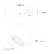
COB 4000 [K] HI EFFICIENT Light colour CRI 90 Led chip flux 3793 [lm] Luminous flux 3034 [lm] System power 23 [W] Luminaire Efficiency 132 [lm/W] Beam angle 20° Controller ON/OFF MacAdam 3 SDCM
