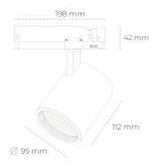
COB 3500 [K] HI EFFICIENT Light colour CRI 90 Led chip flux 1571 [lm] Luminous flux 1256 [lm] System power 10 [W] Luminaire Efficiency 126 [lm/W] Beam angle 20° Controller ON/OFF MacAdam 3 SDCM
