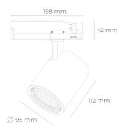
COB 3500 [K] HI EFFICIENT Light colour CRI 90 Led chip flux 3341 [lm] Luminous flux 2672 [lm] System power 21 [W] Luminaire Efficiency 127 [lm/W] Beam angle 15° Controller ON/OFF MacAdam 3 SDCM
