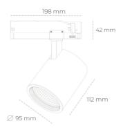
COB 3000 [K] HI EFFICIENT Light colour CRI 90 Led chip flux 4084 [lm] Luminous flux 3267 [lm] System power 25 [W] Luminaire Efficiency 131 [lm/W] Beam angle 30° Controller ON/OFF MacAdam 3 SDCM
