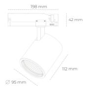
COB 2000 [K] MEAT PINK Light colour CRI Led chip flux 2181 [lm] Luminous flux 1744 [lm] System power 25 [W] Luminaire Efficiency 70 [lm/W] Beam angle 15° Controller ON/OFF MacAdam 3 SDCM
