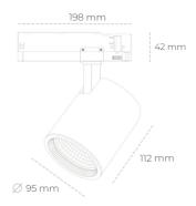
COB 3500 [K] HI EFFICIENT Light colour CRI 90 Led chip flux 1571 [lm] Luminous flux 1256 [lm] System power 10 [W] Luminaire Efficiency 126 [lm/W] Beam angle 15° Controller ON/OFF MacAdam 3 SDCM
