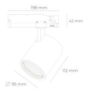
COB 2500 [K] BREAD Light colour CRI Led chip flux 1195 [lm] Luminous flux 956 [lm] System power 10 [W] Luminaire Efficiency 96 [lm/W] Beam angle 60° Controller ON/OFF
