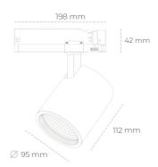
COB 3000 [K] CRI97 Light colour CRI Led chip flux 2601 [lm] Luminous flux 2080 [lm] System power 23 [W] Luminaire Efficiency 90 [lm/W] Beam angle 45° Controller ON/OFF MacAdam 3 SDCM
