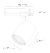
COB 3000 [K] CRI97 Light colour CRI 1144 [lm] Led chip flux Luminous flux 915 [lm] System power 10 [W] Luminaire Efficiency 92 [lm/W] Beam angle 45° Controller ON/OFF MacAdam 3 SDCM
