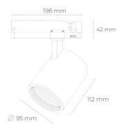
COB 3000 [K] CRI97 Light colour CRI Led chip flux 2601 [lm] Luminous flux 2080 [lm] System power 23 [W] Luminaire Efficiency 90 [lm/W] Beam angle 15° Controller ON/OFF MacAdam 3 SDCM
