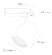
COB 3500 [K] PREMIUM WHITE Light colour CRI 90 Led chip flux 4038 [lm] Luminous flux 3230 [lm] System power 27 [W] Luminaire Efficiency 120 [lm/W] Beam angle 20° Controller ON/OFF MacAdam
