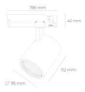
COB 4000 [K] HI EFFICIENT Light colour CRI 90 Led chip flux 3189 [lm] Luminous flux 2551 [lm] System power 19 [W] Luminaire Efficiency 134 [lm/W] Beam angle 60° Controller ON/OFF MacAdam 3 SDCM
