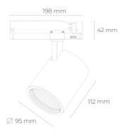
COB 3000 [K] HI EFFICIENT Light colour CRI 90 Led chip flux 1623 [lm] Luminous flux 1298 [lm] System power 10 [W] Luminaire Efficiency 130 [lm/W] Beam angle 30° Controller ON/OFF MacAdam 3 SDCM
