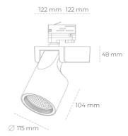
COB 4000 [K] HI EFFICIENT Light colour CRI 90 Led chip flux 2260 [lm] Luminous flux 1808 [lm] System power 14 [W] Luminaire Efficiency 129 [lm/W] Beam angle 60° Controller ON/OFF MacAdam 3 SDCM
