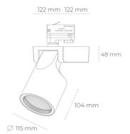
COB 4000 [K] HI EFFICIENT Light colour CRI 90 Led chip flux 1625 [lm] Luminous flux 1300 [lm] System power 10 [W] Luminaire Efficiency 130 [lm/W] Beam angle 30° Controller ON/OFF
