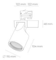
COB 4000 [K] HI EFFICIENT Light colour CRI 90 Led chip flux 3492 [lm] Luminous flux 2793 [lm] System power 21 [W] Luminaire Efficiency 133 [lm/W] Beam angle 20° Controller ON/OFF MacAdam 3 SDCM
