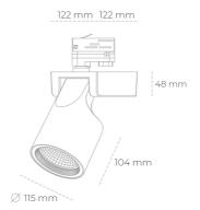
COB 3500 [K] HI EFFICIENT Light colour CRI 90 Led chip flux 1571 [lm] Luminous flux 1256 [lm] System power 10 [W] Luminaire Efficiency 126 [lm/W] Beam angle 60° Controller ON/OFF MacAdam
