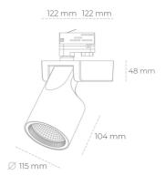
COB 3500 [K] HI EFFICIENT Light colour CRI 90 Led chip flux 4723 [lm] Luminous flux 3778 [lm] System power 31 [W] Luminaire Efficiency 122 [lm/W] Beam angle 20° Controller ON/OFF MacAdam 3 SDCM
