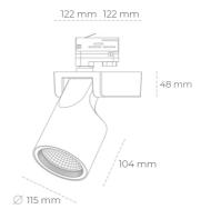
COB 2000 [K] MEAT PINK Light colour CRI 1845 [lm] Led chip flux Luminous flux 1476 [lm] System power 21 [W] Luminaire Efficiency 70 [lm/W] Beam angle 45° Controller ON/OFF MacAdam 3 SDCM
