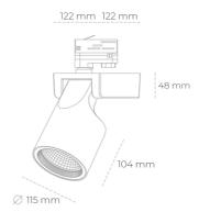
COB 2000 [K] MEAT PINK Light colour CRI 895 [lm] Led chip flux Luminous flux 716 [lm] System power 10 [W] Luminaire Efficiency 72 [Im/W] Beam angle 30° Controller ON/OFF MacAdam 3 SDCM
