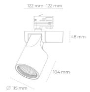
COB 5700 [K] SPECIAL Light colour CRI Led chip flux 1318 [lm] Luminous flux 1054 [lm] System power 10 [W] Luminaire Efficiency 105 [lm/W] Beam angle 30° Controller ON/OFF
