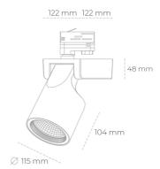
COB 4200 [K] MEAT WHITE Light colour CRI 90 Led chip flux Luminous flux 818 [lm] System power 10 [W] Luminaire Efficiency 82 [lm/W] Beam angle 20° Controller ON/OFF MacAdam 3 SDCM
