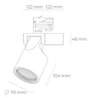
COB 4000 [K] HI EFFICIENT Light colour CRI 90 Led chip flux 3189 [lm] Luminous flux 2551 [lm] System power 19 [W] Luminaire Efficiency 134 [lm/W] Beam angle 20° Controller ON/OFF MacAdam 3 SDCM
