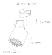
COB 3000 [K] HI EFFICIENT Light colour CRI 90 Led chip flux 4378 [lm] Luminous flux 3502 [lm] System power 27 [W] Luminaire Efficiency 130 [lm/W] Beam angle 45° Controller ON/OFF MacAdam 3 SDCM
