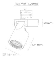
COB 2000 [K] MEAT PINK Light colour CRI 1845 [lm] Led chip flux Luminous flux 1476 [lm] System power 21 [W] Luminaire Efficiency 70 [lm/W] Beam angle 45° Controller ON/OFF
