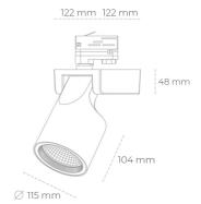
COB 3000 [K] CRI97 Light colour CRI 3368 [lm] Led chip flux Luminous flux 2694 [lm] System power 31 [W] Luminaire Efficiency 87 [lm/W] Beam angle 45° Controller ON/OFF MacAdam 3 SDCM
