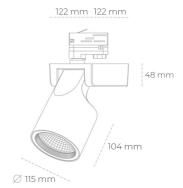
COB 3000 [K] CRI97 Light colour CRI Led chip flux 2601 [lm] Luminous flux 2080 [lm] System power 23 [W] Luminaire Efficiency 90 [lm/W] Beam angle 20° Controller ON/OFF MacAdam 3 SDCM
