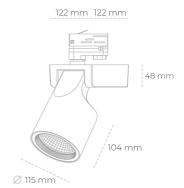
COB 5700 [K] SPECIAL Light colour CRI 3934 [lm] Led chip flux Luminous flux 3147 [lm] System power 31 [W] Luminaire Efficiency 102 [lm/W] Beam angle 60° Controller ON/OFF
