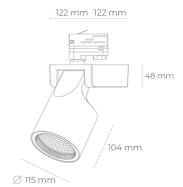
COB 5700 [K] SPECIAL Light colour CRI 3023 [lm] Led chip flux Luminous flux 2418 [lm] System power 23 [W] Luminaire Efficiency 105 [lm/W] Beam angle 30° Controller ON/OFF
