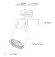
COB 4200 [K] MEAT WHITE Light colour CRI 90 Led chip flux 1976 [lm] Luminous flux 1580 [lm] System power 19 [W] Luminaire Efficiency 83 [lm/W] Beam angle 15° Controller ON/OFF MacAdam 3 SDCM
