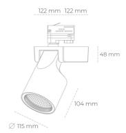
COB 4000 [K] HI EFFICIENT Light colour CRI 90 Led chip flux 1625 [lm] Luminous flux 1300 [lm] System power 10 [W] Luminaire Efficiency 130 [lm/W] Beam angle 20° Controller ON/OFF MacAdam 3 SDCM
