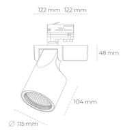
COB 3000 [K] HI EFFICIENT Light colour CRI 90 Led chip flux 3487 [lm] Luminous flux 2789 [lm] System power 21 [W] Luminaire Efficiency 133 [lm/W] Beam angle 45° Controller ON/OFF MacAdam 3 SDCM
