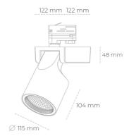
COB 3000 [K] HI EFFICIENT Light colour CRI 90 Led chip flux 2256 [lm] Luminous flux 1804 [lm] System power 14 [W] Luminaire Efficiency 129 [lm/W] Beam angle 45° Controller ON/OFF MacAdam 3 SDCM
