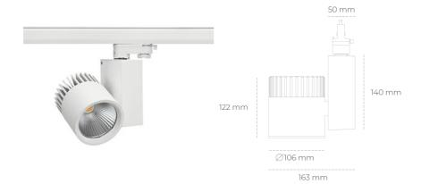
COB Light colour 2000 [K] MEAT PINK CRI Led chip flux 2495 [lm] Luminous flux 1996 [lm] System power 31 [W] Luminaire Efficiency 64 [lm/W] Beam angle 60° Controller ON/OFF MacAdam 3 SDCM
