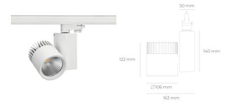
COB Light colour 2000 [K] MEAT PINK CRI Led chip flux 2495 [lm] Luminous flux 1996 [lm] System power 31 [W] Luminaire Efficiency 64 [lm/W] Beam angle 45° Controller ON/OFF MacAdam 3 SDCM
