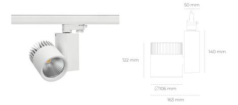
COB Light colour 2000 [K] MEAT PINK CRI Led chip flux 2013 [lm] Luminous flux 1610 [lm] System power 23 [W] Luminaire Efficiency 70 [lm/W] Beam angle 45° Controller ON/OFF MacAdam 3 SDCM
